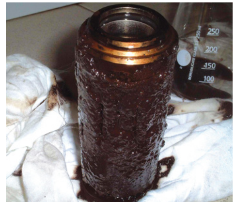
An oil filter from a gas turbine system plugged with sludge. Regular high velocity oil flushing can help keep varnish and sludge under control, but if a filter has already plugged or failed, a high-velocity oil flush may be needed to remove all the debris released into the oil system.
